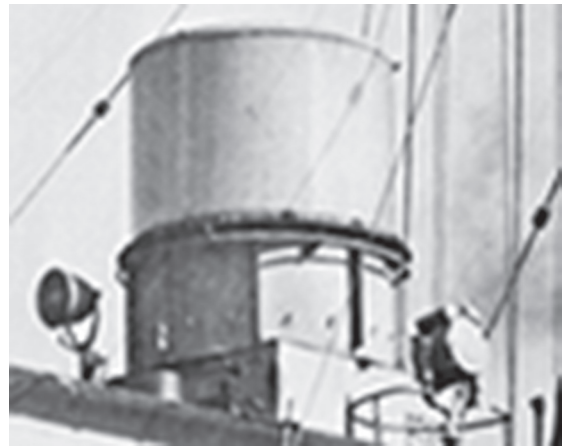
32 A Type 30 (Naval Type 273) Perspex lantern mounted on a ship, but identical to the lantern used at Naval CDU stations.
