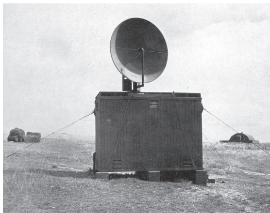
33 A Type 31 radar as usually deployed, in its transportable wooden cabin.
