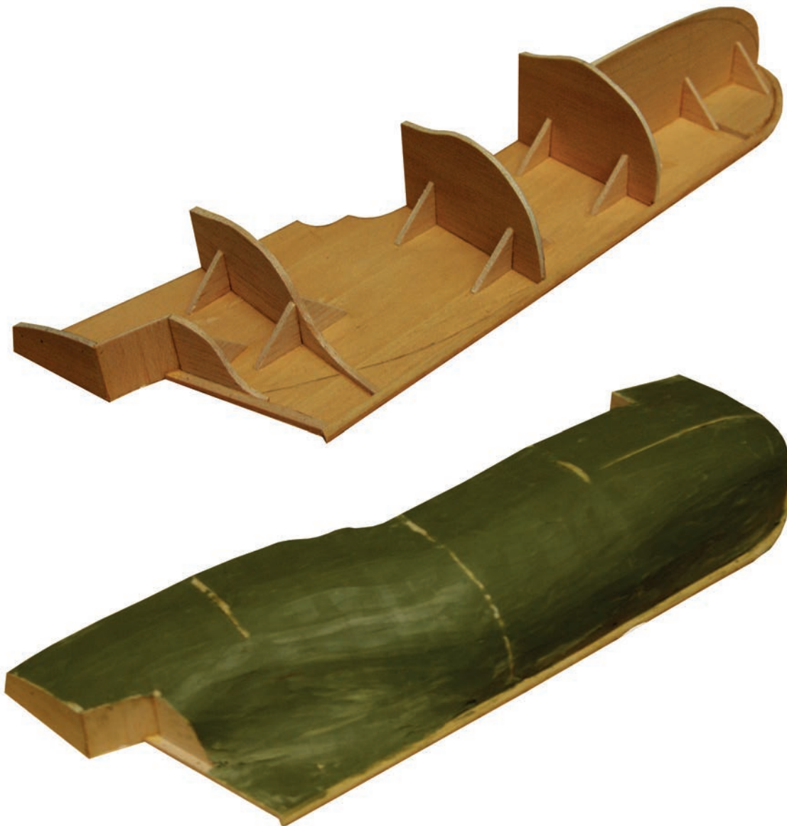
Illustration 132 Top: speculative framework of the hull based on recorded elements. Bottom: speculative half-model faired with modelling-compound
