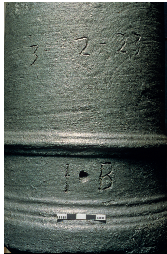
Illustration 202 Surface detail of Gun 8 [82] at the breech, showing the initials of John Browne of Horsmonden and the weight in hundredweights, quarters, and pounds. These marks were cut with a chisel after casting. Note the marks which represent a final wiping of the clay surface of the mould pattern. Scale in centimetres (DP 174286)
