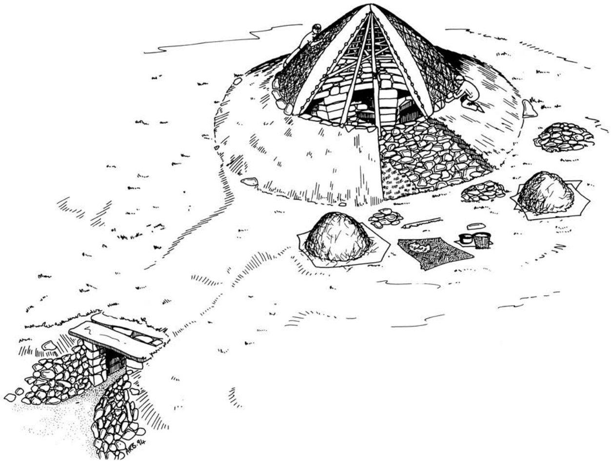
ILLUSTRATION 5.4(b) Wheelhouse construction: Drawing Four.
