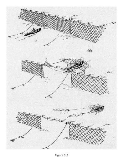
How indicator nets work: (top) the submerged submarine approaches the moored net; (middle) the submarine hits the net and the clips holding the net sections together part; (bottom) the 'pram buoys', filled with phosphate of carbide, burn on the surface, showing the location and course of the submarine (US Bureau of Ordnance 1944 Net and Boom Defenses)
