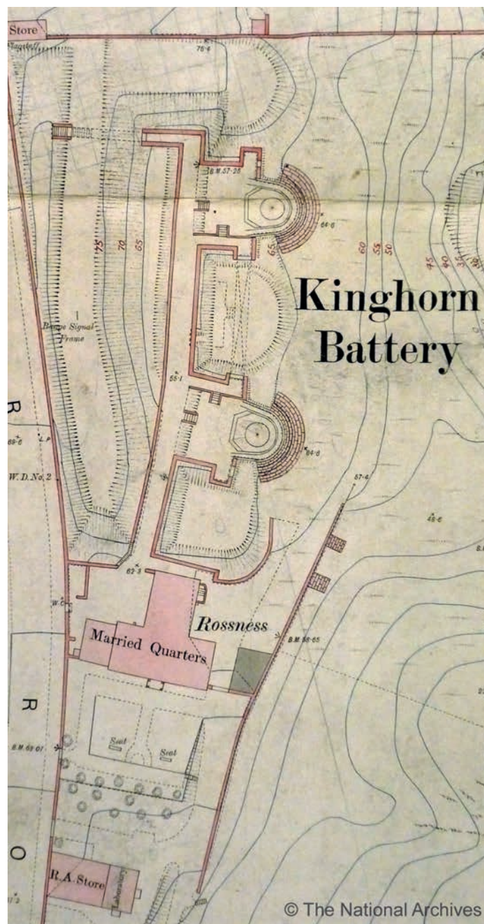
Figure 11.69 Detail of a large-scale plan of the Kinghorn Battery, drawn in 1890 (© The National Archives, WO 78/4173)
