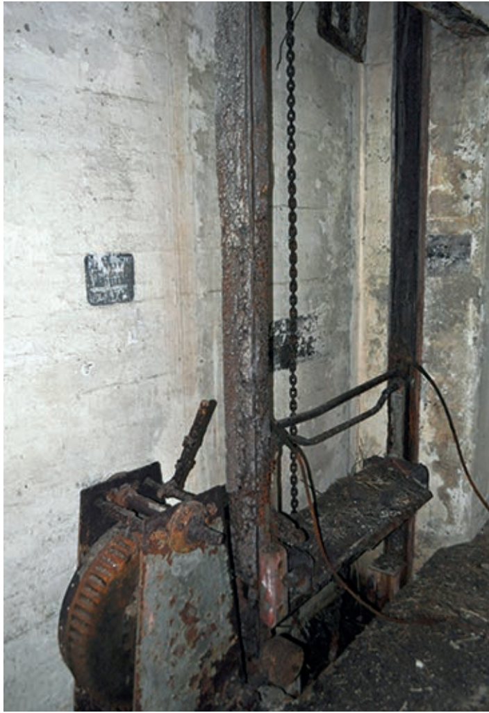
Figure 11.24 The quick-return lift of the mid-9.2-inch gun (© Gordon Barclay)
